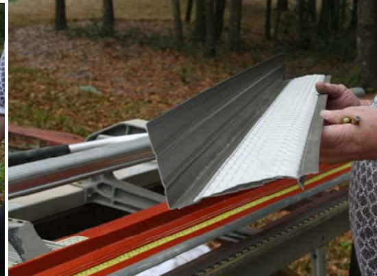
Field forming for fascia mount applications using a small sheet metal hand brake
